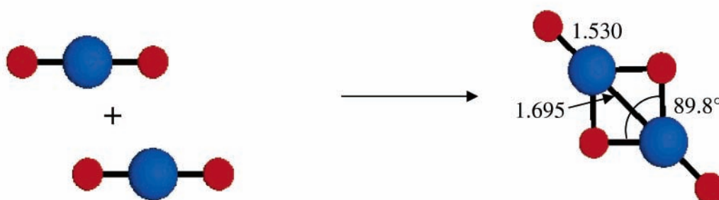
Figure 2. The lowest-energy \text{Si}_2\text{O}_3 isomers; MP2/6-31G(d) geometry parameters (Å).
